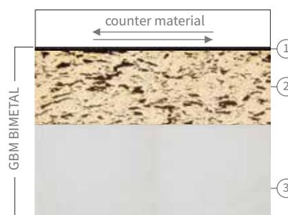
1. SLIDING SURFACE optionally with running-in film applied
